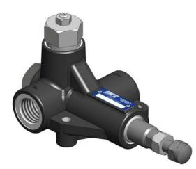
Push button valve designed for the use on trailers and semi-trailers to stop the run of tipper cylinders. The valve is normally closed, is mounted on the cylinder and diverts the oil to drain when operated by the cylinder itself. An antishock valve is also present to avoid damages on the cylinder.
