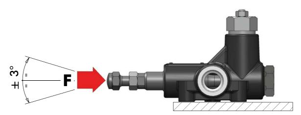
**PS.** The working force  $\mathbf{F}$  has to be higher than  $15 + p \times 3.8$ , where p is the oil pressure in bar.
